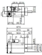
① Encoder connecto 2 Motor connector
